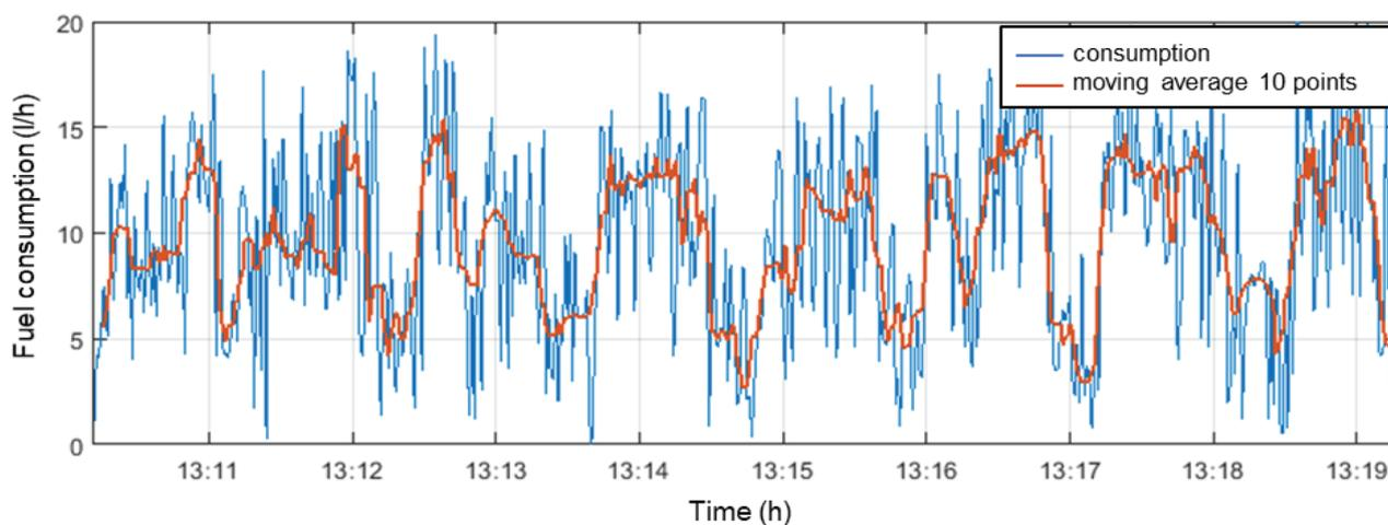
**Figure 4.** Tractor fuel consumption values (l/h), collected over time.
