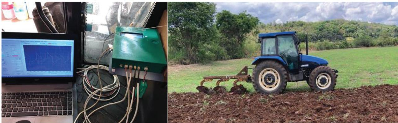
**Figure 3.** Automatic data collection system-ADAS/SIAD embedded in the tractor + implement set (TL-95E New Holland and moldboard plow, 3x28'') in field tests.
