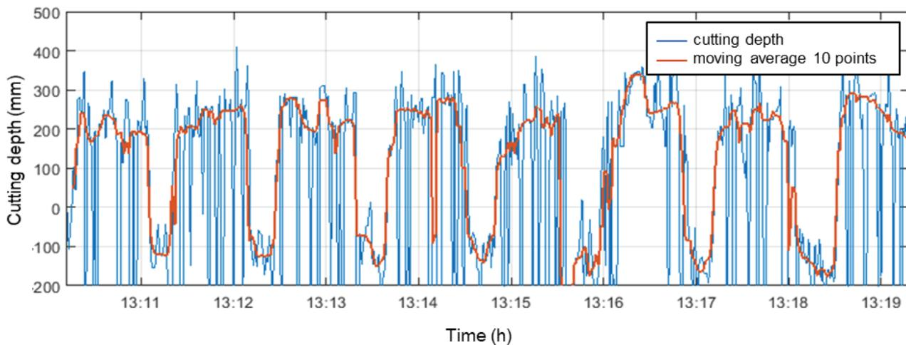
**Figure 7.** Moldboard plow cutting depth (mm) over time.
