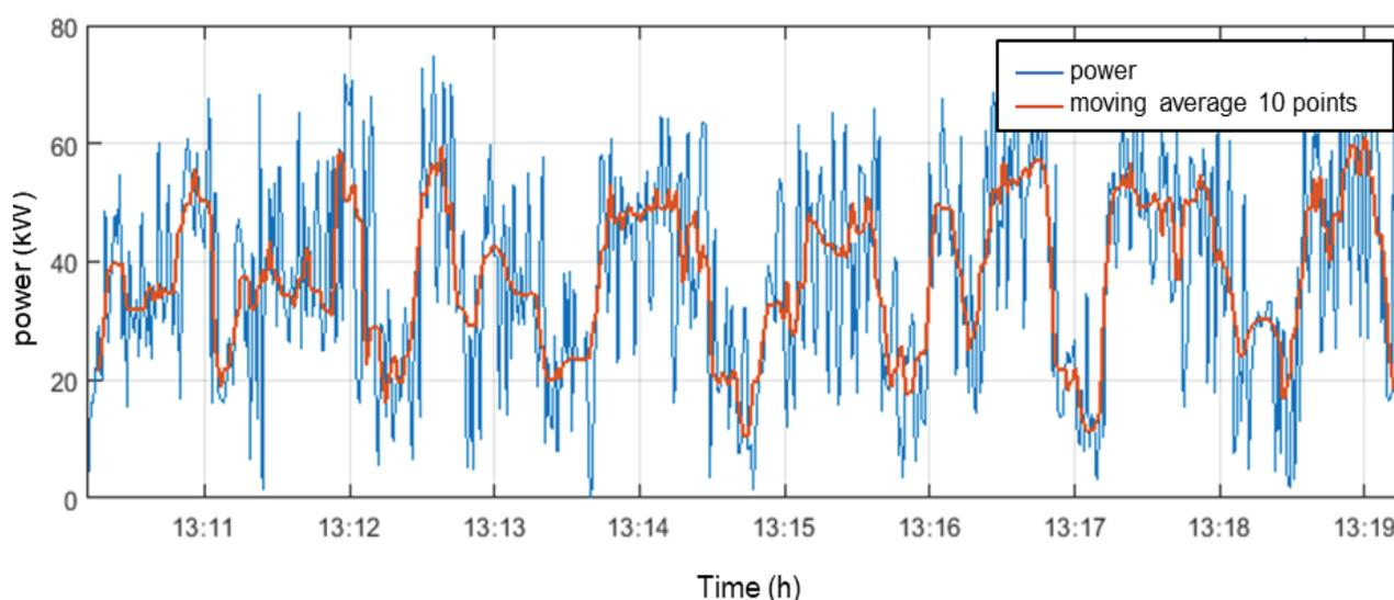
**Figure 9.** Power (kW) demanded by the implement, over time.
