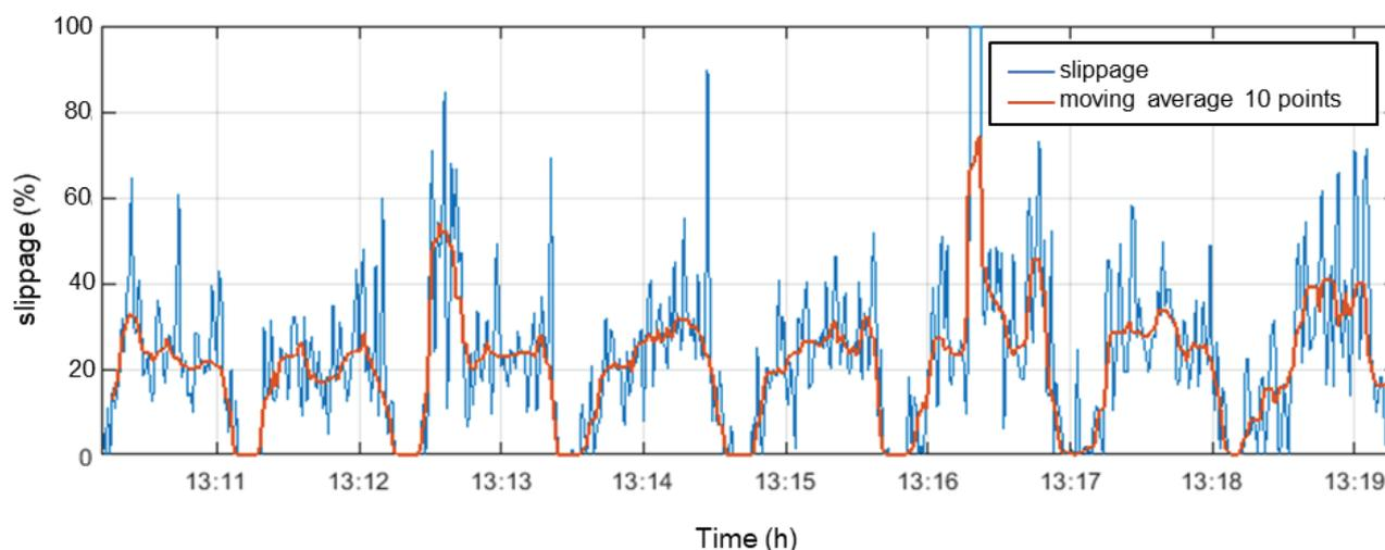
**Figure 8.** Tractor drive wheel slippage (%) over time.
