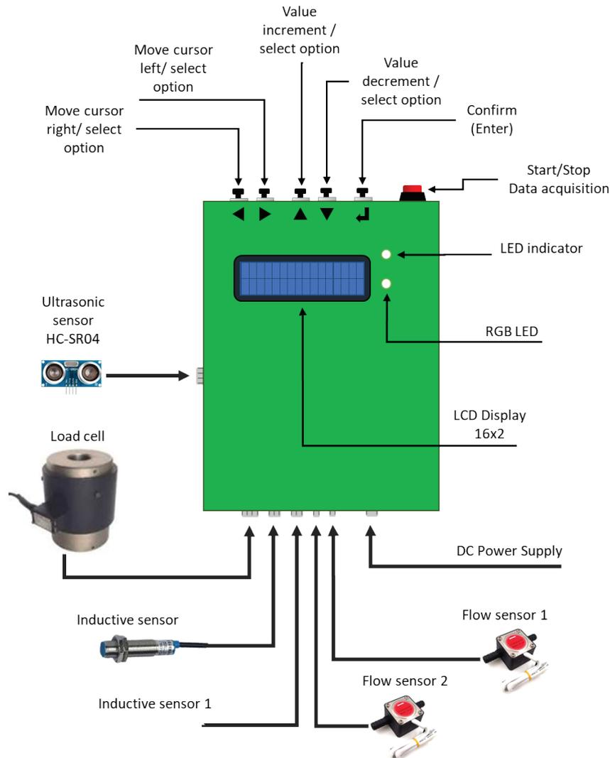
**Figure 1.** Overview of the developed ADAS/SIAD, with the respective sensors and user interface components (buttons and display).
