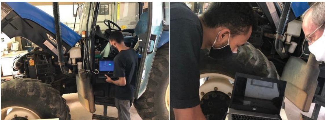
**Figure 2.** Automatic data acquisition system-ADAS/SIAD (data collector) and tests in the Mechanization Laboratory of the tractor-implement set (TL-95E New Holland and moldboard plow, 3x28”), of adjustments/calibration of the signals of each sensor, prior to field testing.
